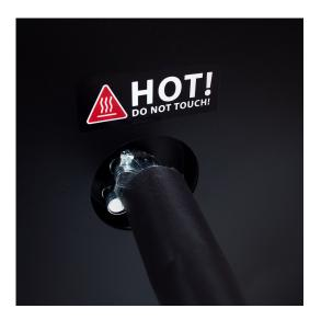
It is possible to connect a 60mm air duct to the hot air outlet and air inlet. To connect the 60mm air duct to the air intake, remove the plastic cover from the air intake, by screwing it ½ counterclockwise and removing the grill.
